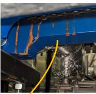
High pressure water leaked into the atmospheric silicone oil side
